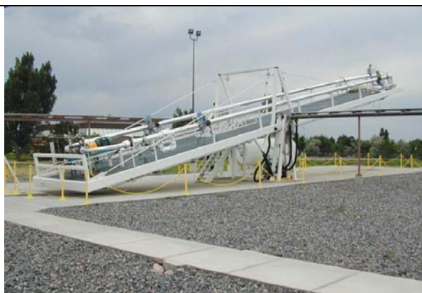
Figure 2: Flow Assurance Loop Mounted on Tilt Table
